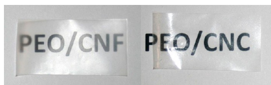
Figure 3. PEO/CNF and PEO/CNC nanocomposite films at room temperature. CNF and CNC concentration: 7%.
